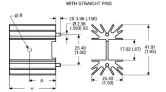
A Dim 18.29 (.720) B Dim 3.18 (.125) H Dim 38.1 (1.50)
